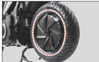
Abb. 26 Motor (Hinterrad)
