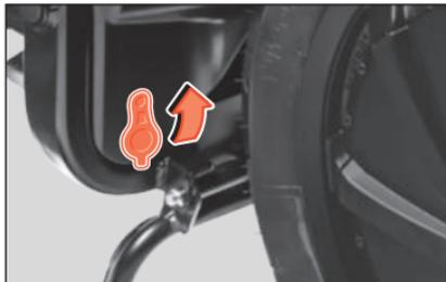
Fig. 32 Left side of the eScooter: safety latch
