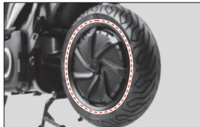
Fig. 26 Motor (rear wheel)
