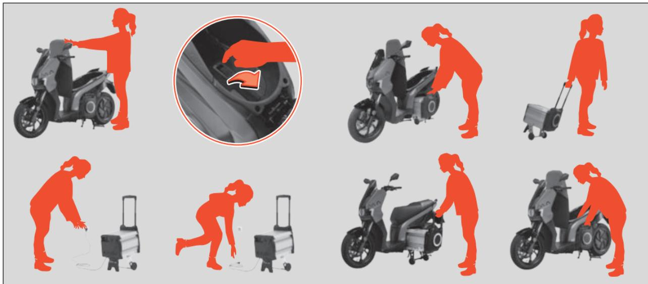
**Fig. 31** Removing the battery
