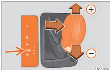
Abb. 102 Hebel in Tiptronic-Stellung.
